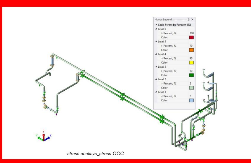
CONCLUSIONS Giorgi Engineering supplied the expansion compensators, flexible hoses and variable load elastic supports required to absorb the line's expansion.
