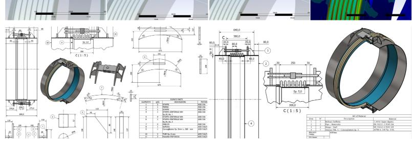
CHALLENGE The main challenge was choosing a special combination of geometry and material for angular mechanism to resist the moments, forces and finally different types of stresses that created in the requested pressure, temperature, and diameter of the compensator.
